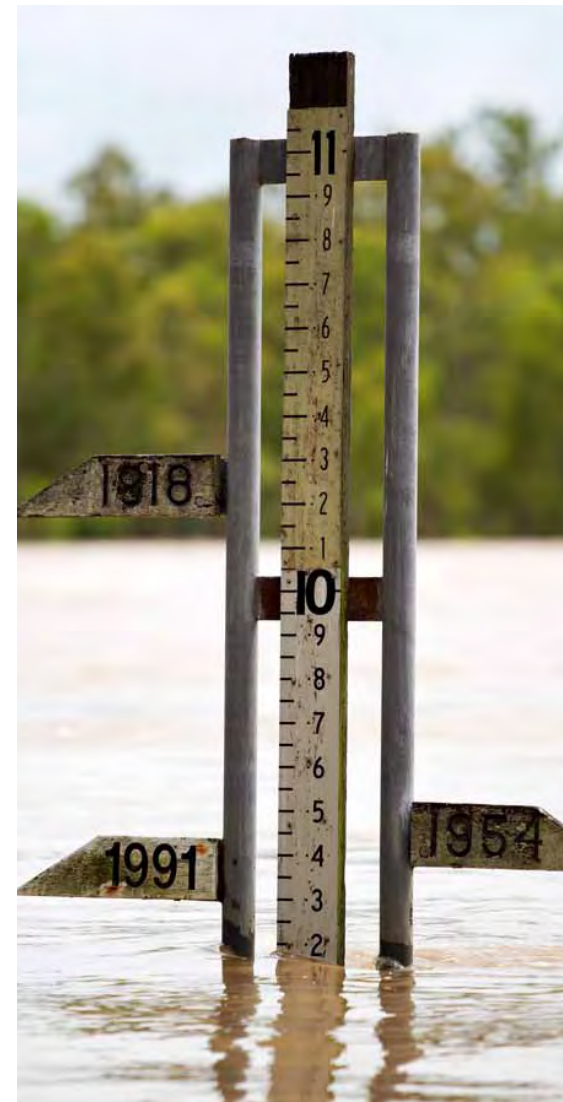
Photo: A manual stream gauging station on the Fitzroy River, Rockhampton, January 2011. Note the historical reference to heights of previous floods: 1918, 1954 and 1991. Photographer: Michael Marston
