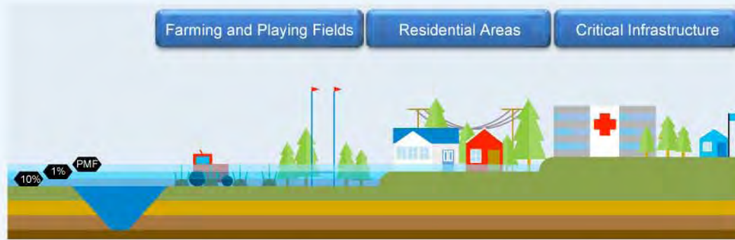
Figure 13. Land use planning should consider flood behaviour and risk. Probable Maximum Flood (PMF) is an estimation of the largest possible flood that could occur at a particular location. Critical public infrastructure such as hospitals and emergency management centres are ideally located outside the influence of the PMF. From Q6 we note that a 10% flood is a ‘1 in 10-year flood’ and a 1% flood is a ‘1 in 100-year flood’. Courtesy of WMAwater.
