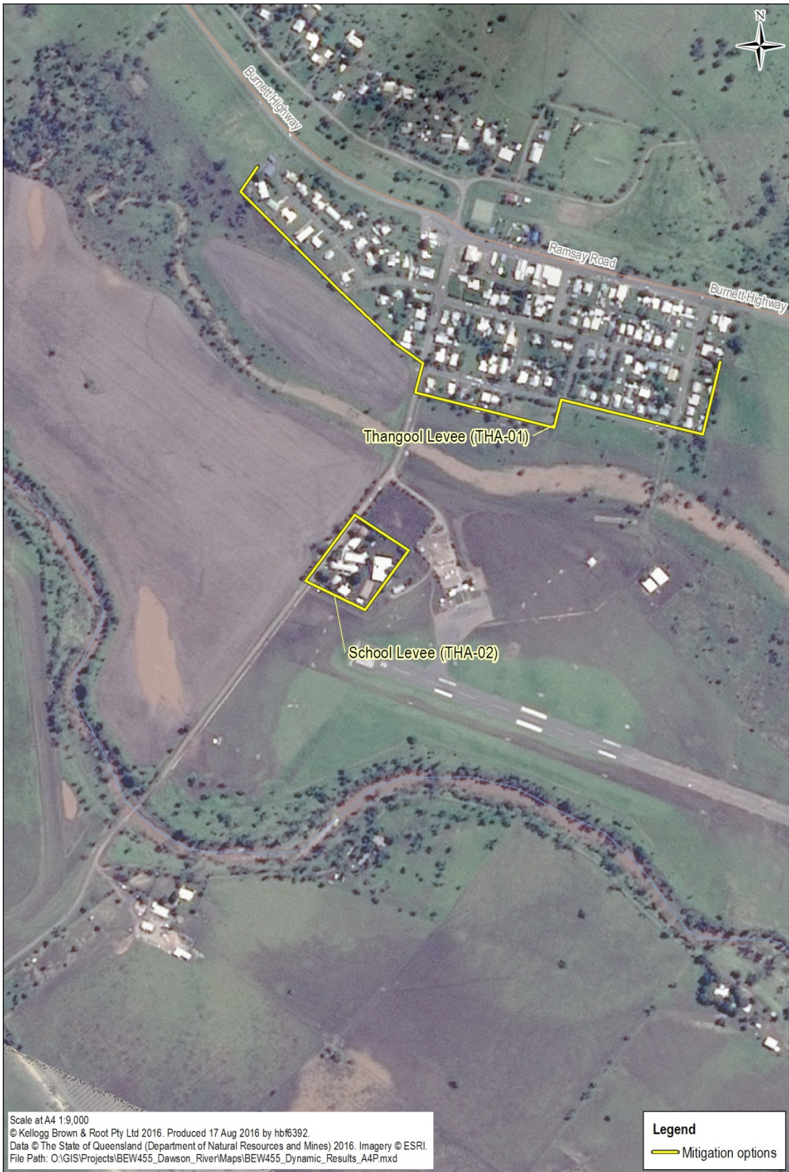
Figure 4.1 POTENTIAL STRUCTURAL MITIGATION AT THANGOOL
