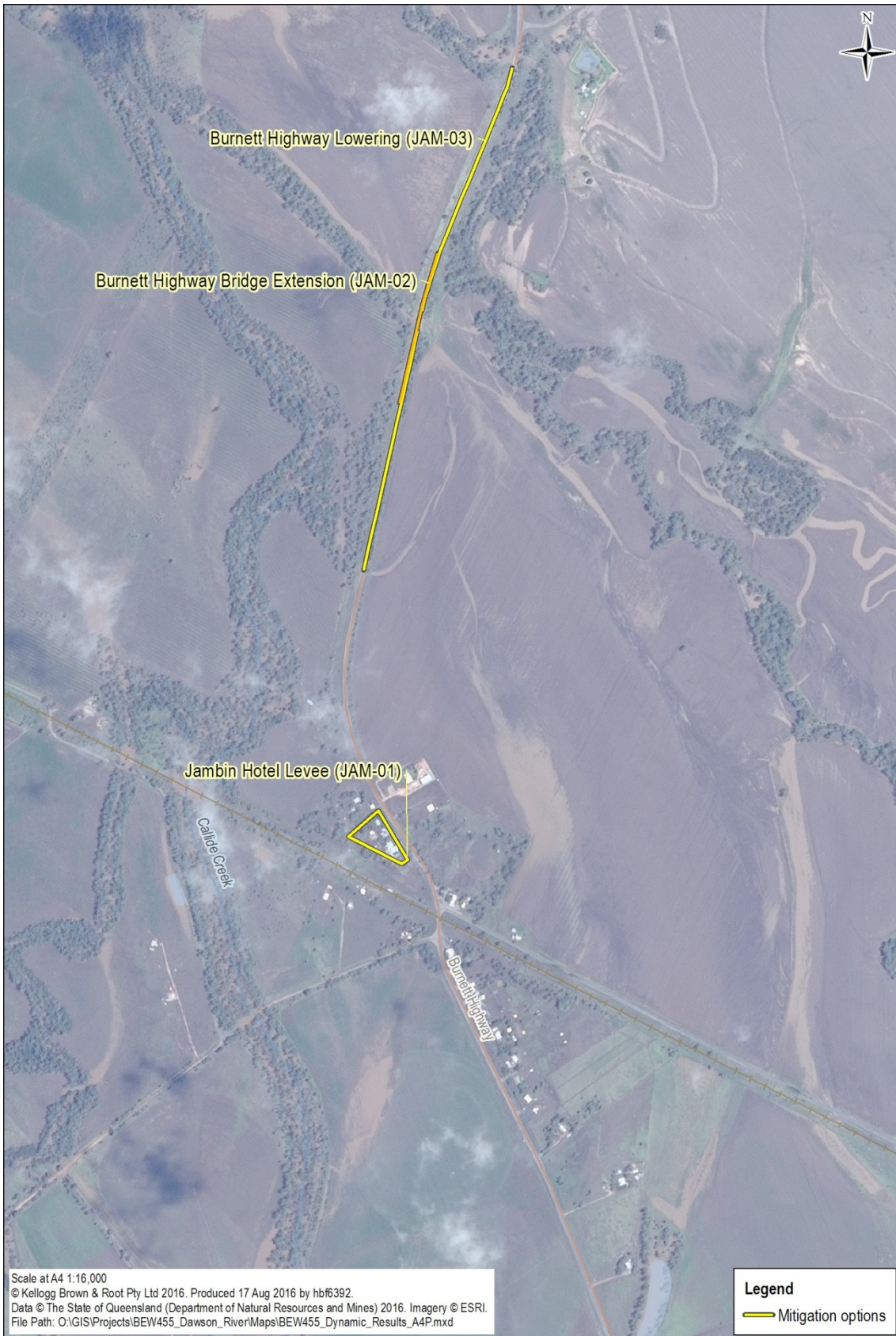
Figure 4.4 POTENTIAL STRUCTURAL MITIGATION OPTIONS IN JAMBIN
