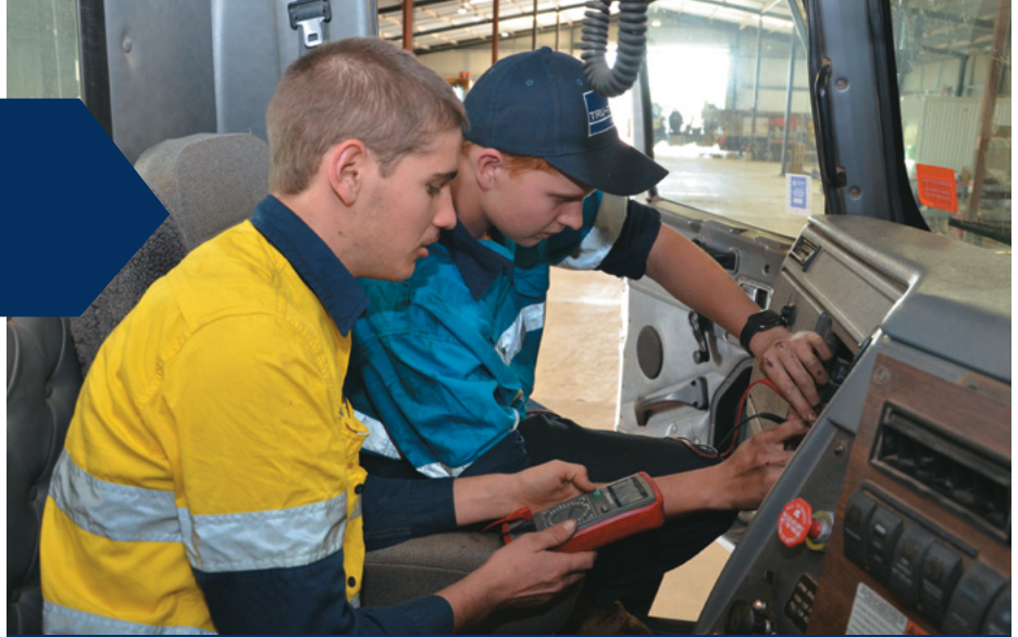
Apprentice diesel fitter Cameron Smith and school-based apprentice diesel fitter Matthew Davidson attempting to locate a fault in the Western Star semi-trailer
