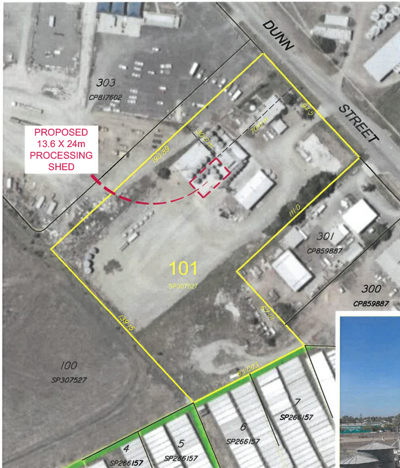
PROPOSED PROCESSING SHED GROSS FLOOR AREA - 326 m
