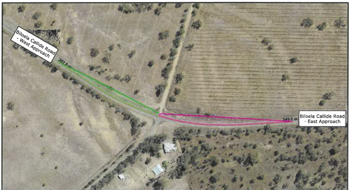
Figure 2-9 Biloela Callide Road / Shorts Road / Linkes Road intersection – Shorts Road approach safe intersection sight distances
