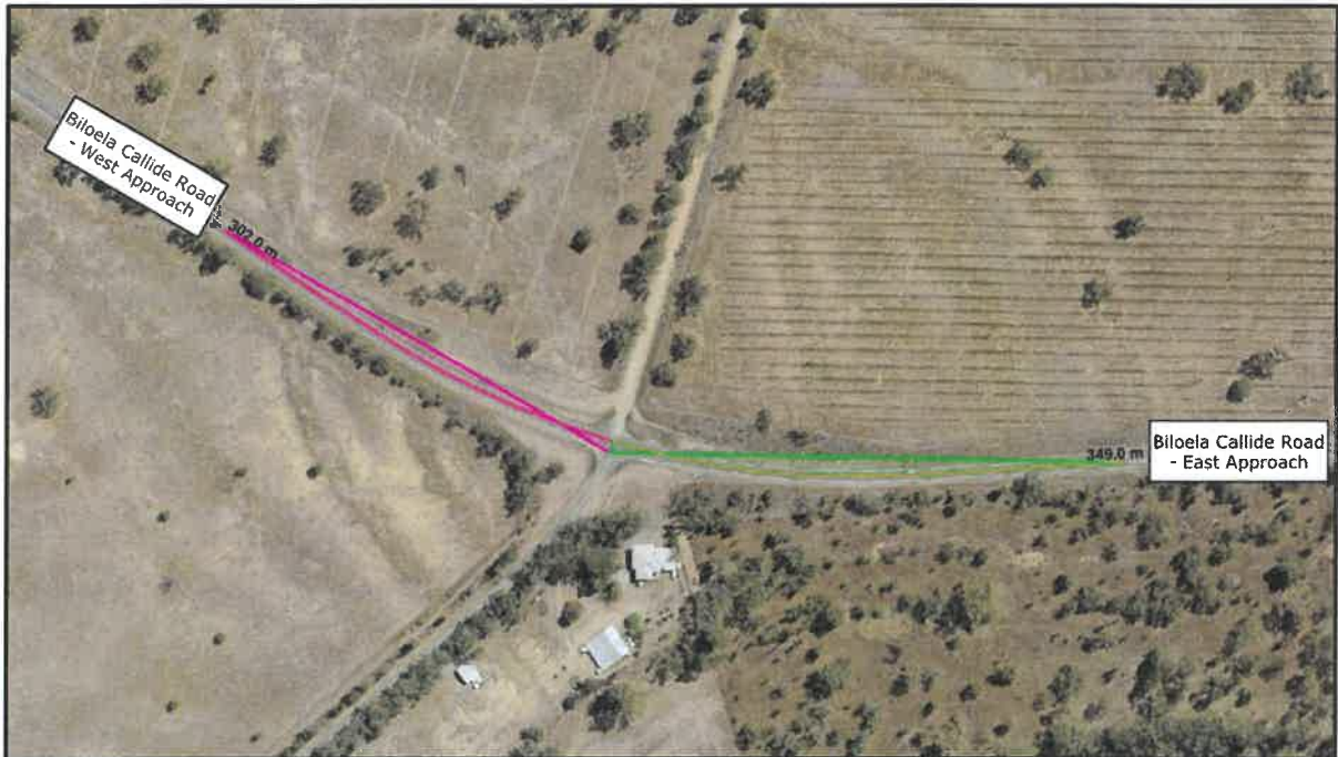
Figure 2-8 Biloela Callide Road / Shorts Road / Linkes Road intersection – Linkes Road approach safe intersection sight distances
