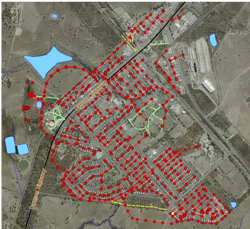
Figure 5: Moura Sewer Network
