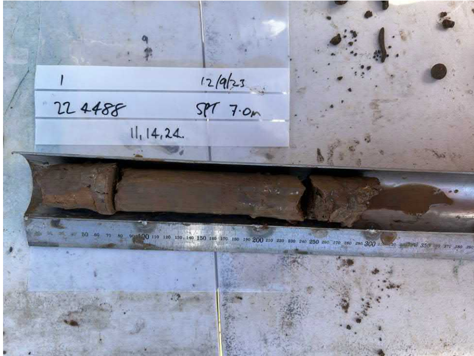
Bore 1 – SPT 7.0m
