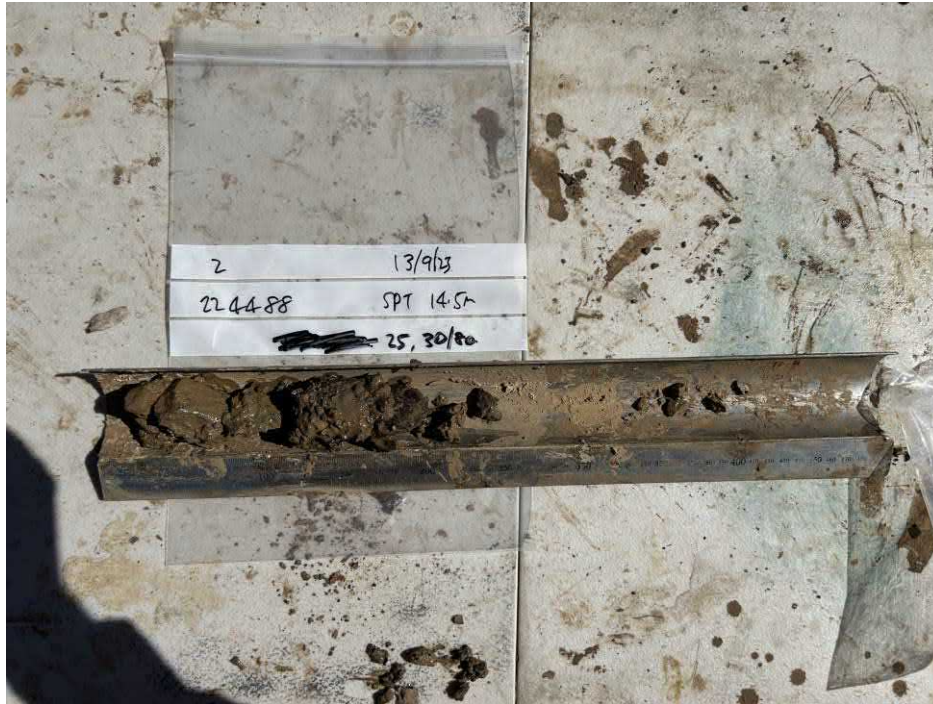
Bore 2 – SPT 14.5m
