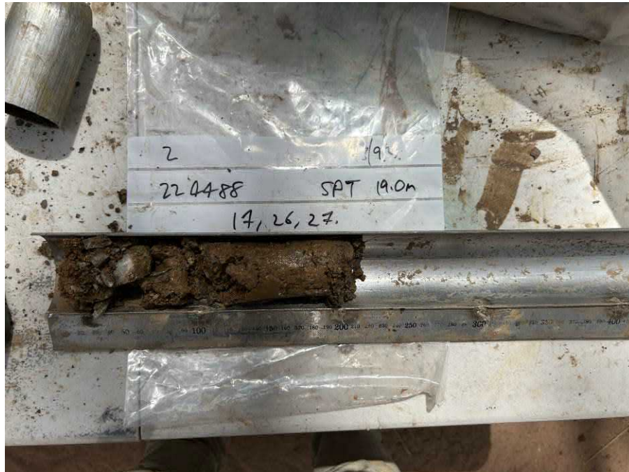
Bore 2 – SPT 19.0m
