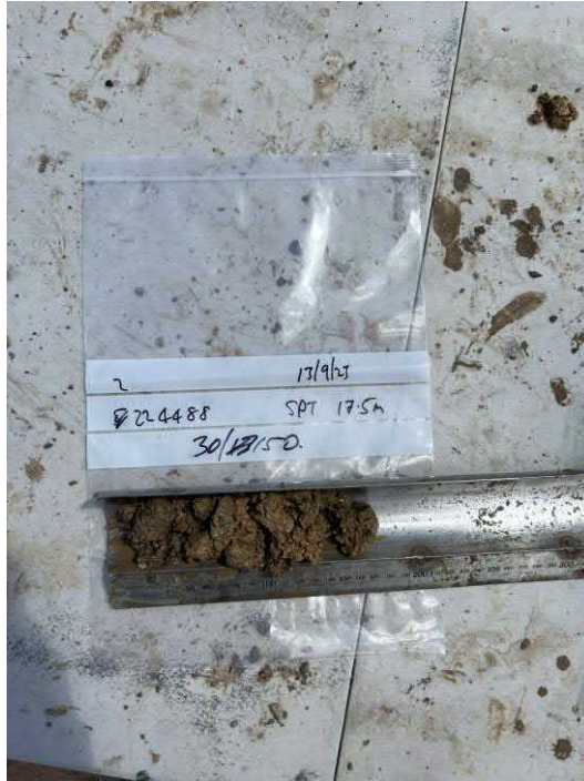
Bore 2 – SPT 17.5m
