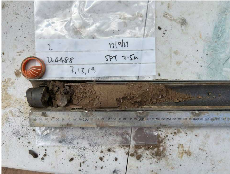
Bore 2 – SPT 2.5m
