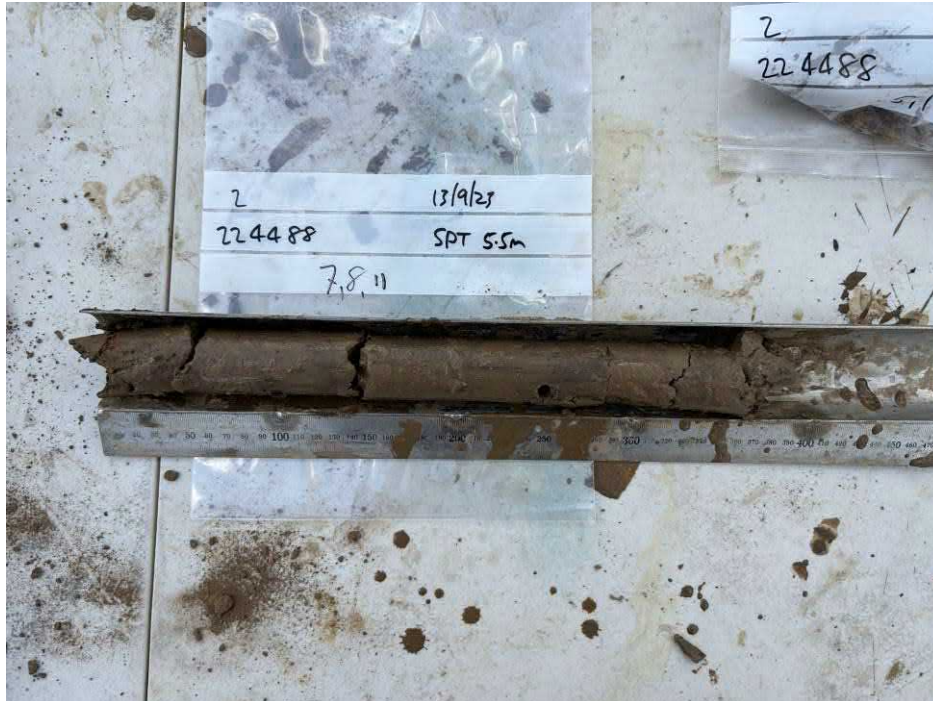
Bore 2 – SPT 5.5m
